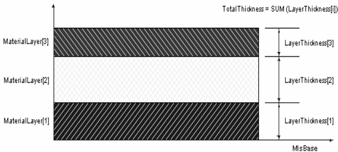
Figure 9: The multi-layering system of materials in IFC
